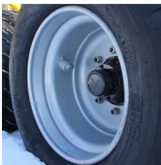
Reinforced wheels with valve protection
