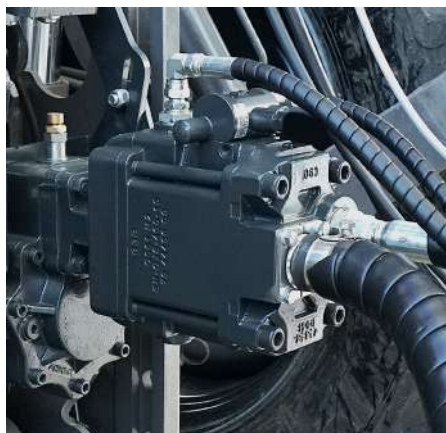
Piston pump & multiplier in PTO
