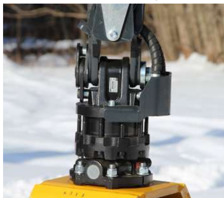
Rotator with hose protection cover
