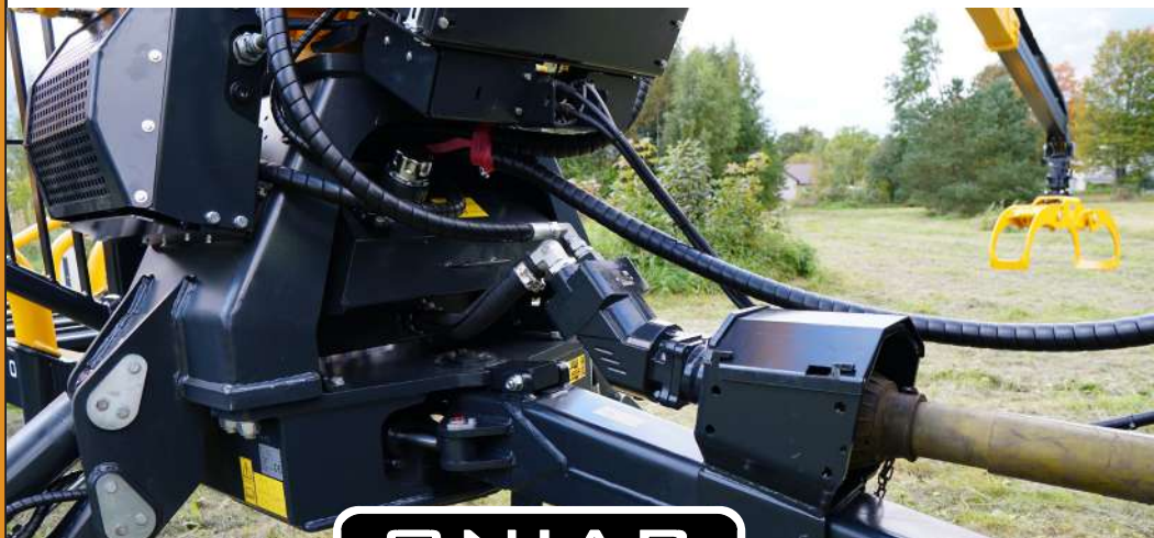
Piston pump & multiplier in PTO
