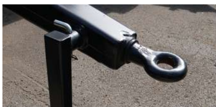
Welded swivel towing eye Ø 50 mm
