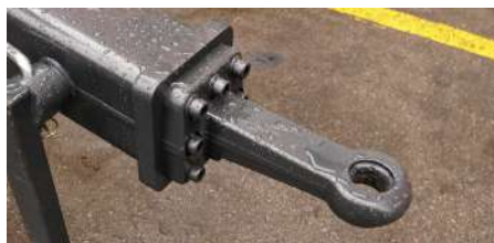
Bolted fix towing eye Ø 40 mm
