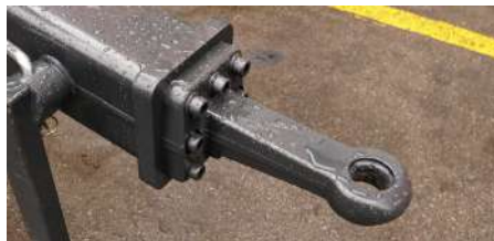
Bolted fix towing eye Ø 40 mm
