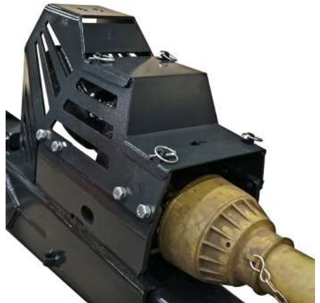
Protected piston pump & multiplier on drawbar
