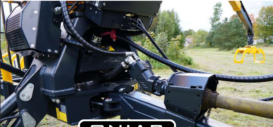
Piston pump & multiplier in PTO
