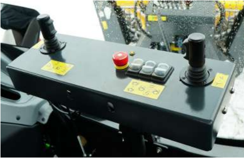
Valve block full electric with mini joysticks FIX / LS
