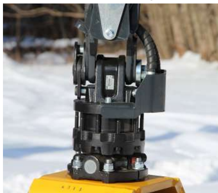
Rotator with hose protection cover
