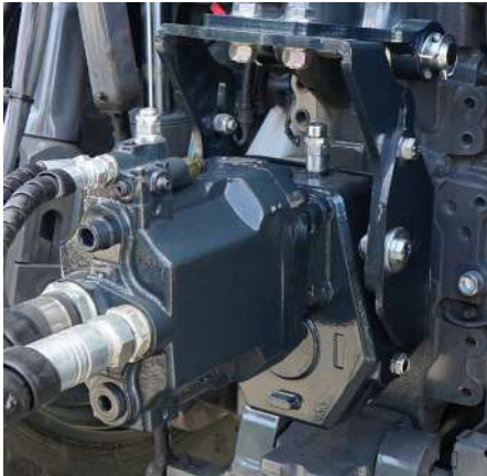
Piston pump & multiplier in PTO
