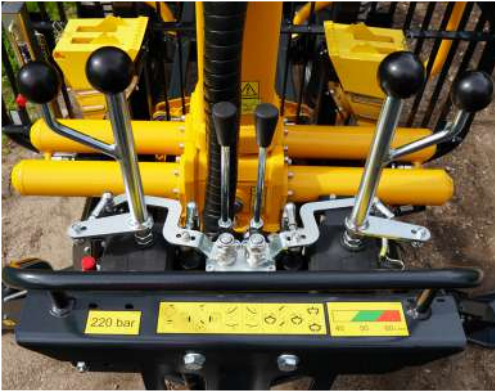
Valve block 4/8 XYZ control
