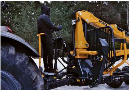
Standing platform for control valve on drawbar with pump connection underneath
