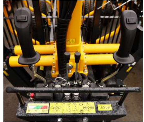
Valve block 4/8 XY control ON-OFF
