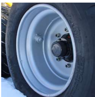
Reinforced wheels with valve protection
