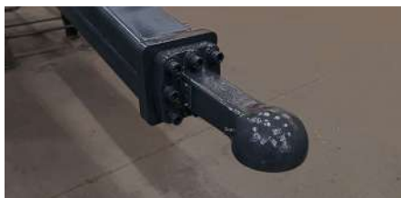
Fix towing eye ball coupling Ø 80mm
