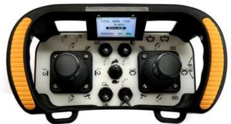
Battery operated radio remote control (hall effect joysticks) allows to operate crane either from tractor cabin or next to crane. Remote control is light, compact and available with two speed settings
