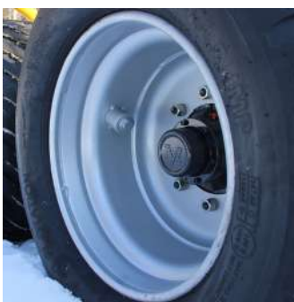
Reinforced wheels with valve protection
