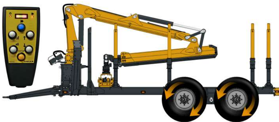
Driving system with Black Bruin motors 2WD / 4WD
