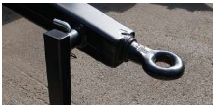
Welded swivel towing eye Ø 50 mm
